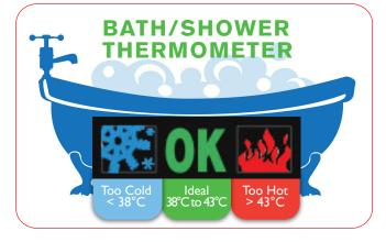
Instructions for Use: Hold the Bath/Shower Thermometer Card in the bath/shower water for 10 seconds. A picture on the black strip on the front of the card will show the temperature of the water. The "OK" picture must show to go on with the bath/shower.
